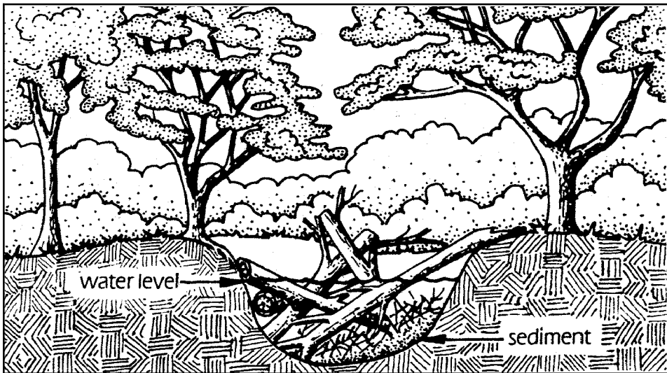
Exhibit 5.4c: Illustration of a Condition 3 Logjam (Source: American Fisheries Society Obstruction Removal Guidelines)
